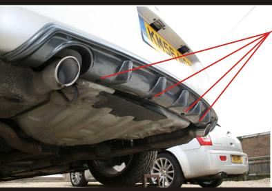
Locate diffuser to underside of bumper holding firm whilst locating and securing original fixings through diffuser.
