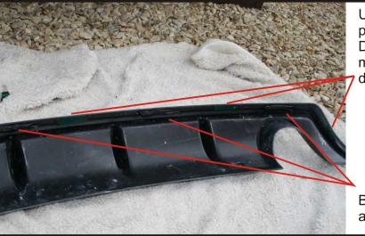
Use strips of 3m type double sided moulding tape placed at regular intervals along outside lip edge. Dependant on tape thickness 1, 2 or 3 levels of tape may be required to 'pad' out proud of the lip on the diffuser.
